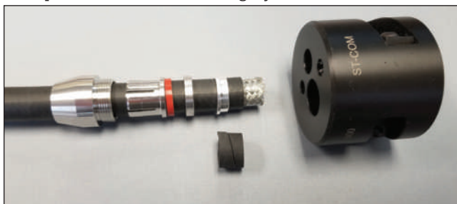
▲ Fig. 2 Prepping the TCOM cable for the connector.
