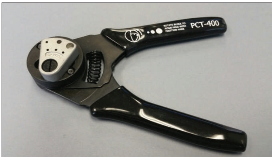
▲ Fig. 3 One of the tools used to replace a connector in the field.
